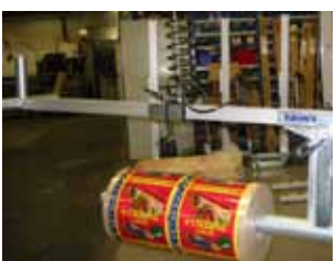
An outbalanced boom for reel lifting.
